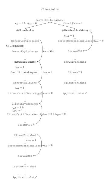
Fig. 3. State machine for commonly used TLS configurations: Protocol versions v = TLSv1.0|TLSv1.1|TLSv1.2. Key exchanges kx = RSA|DHE|ECDHE. Optional feature flags: resumption using server-side caches  $(r_{id})$  or tickets  $(r_{tick})$ , client authentication  $(c_{ask}, c_{offer})$ , new session ticket  $(n_{tick})$ .
