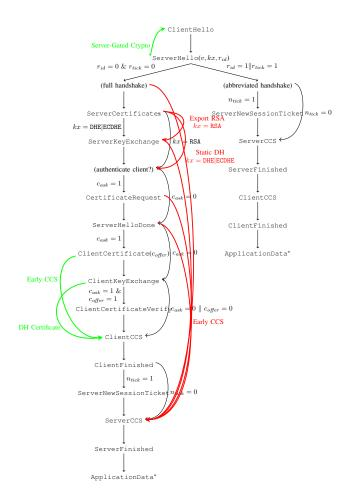
Fig. 5. OpenSSL Client and Server State machine for HTTPS configurations. Unexpected transitions: client in red on the right, server in green on the left
