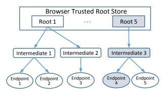
Fig. 1. Web PKI example, depicting trust chain from Root 5 to Endpoint 4.
